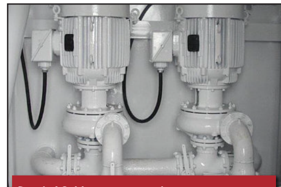
Dual 60 Horsepower electric mix motors
